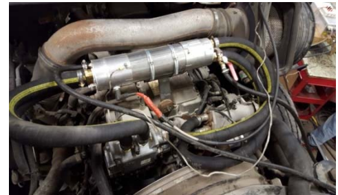
Paradigm Plasma Reactor installed in EGR of a 13.1 L Diesel Engine
